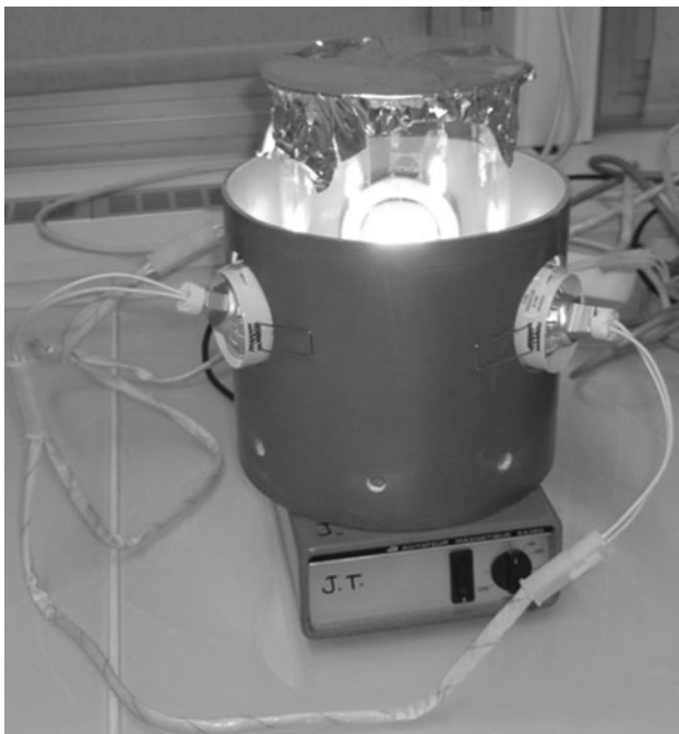
Fig. 3 Photobioreactor. Cells were grown in the bottle sitting in the core of the photosystem with the three LEDs
